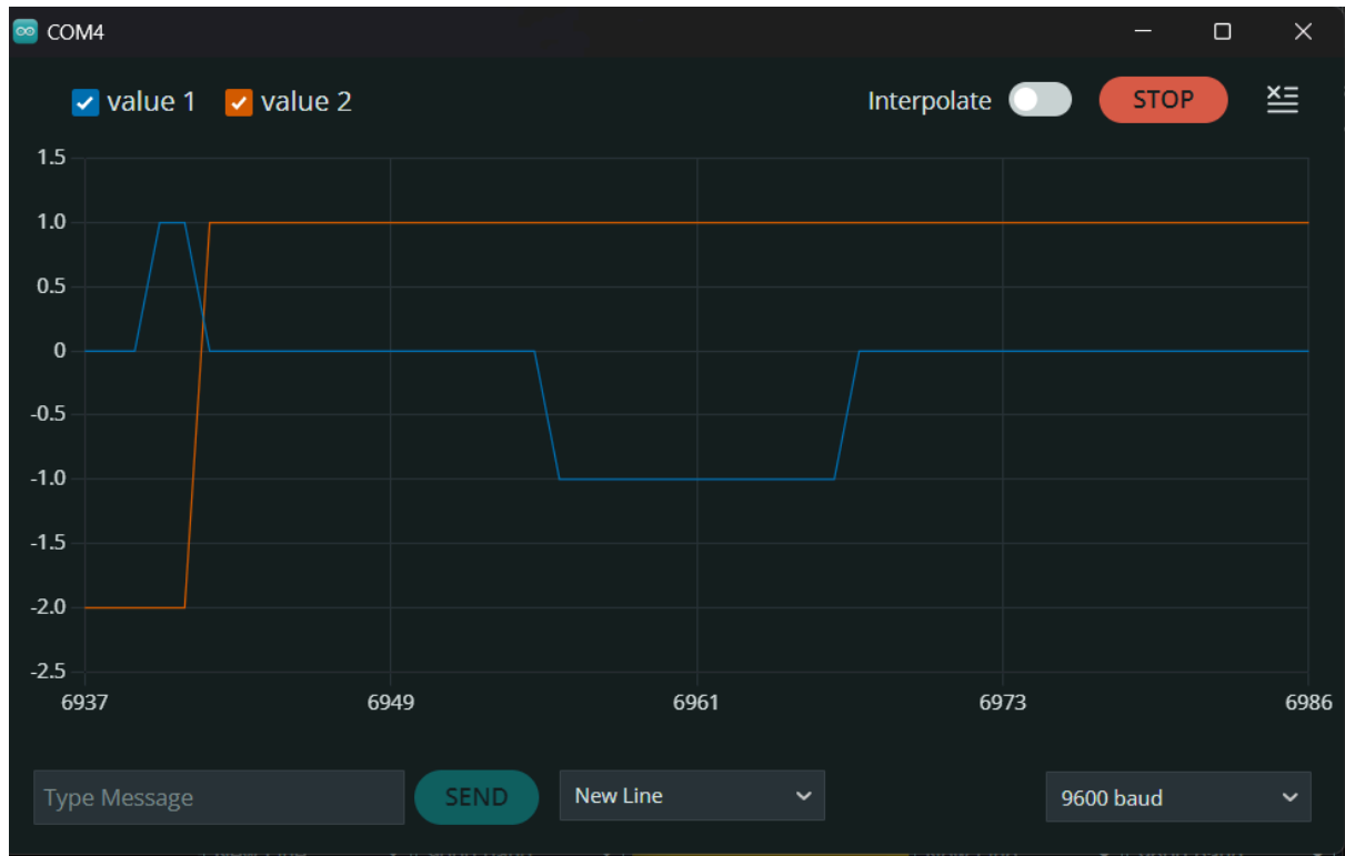
Figure 11.2 Performance with PID controller (Blue is angle, Red is stepper response)
