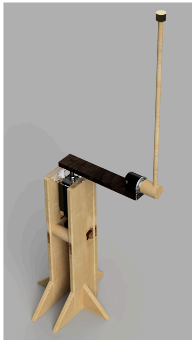
Figure 7.1: Fusion 360 Drawing of Inverted Pendulum Assembly Render
