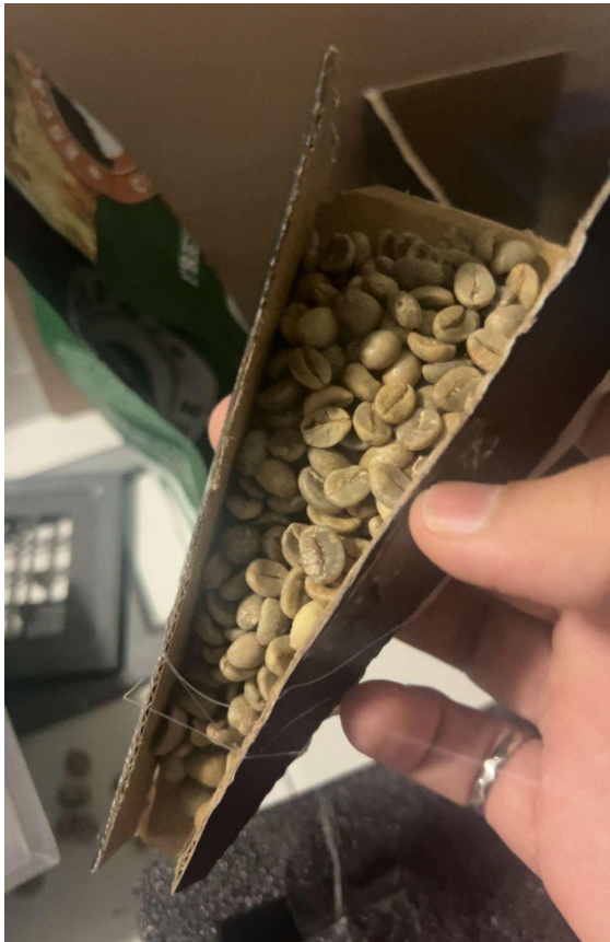
Figure 10.12 - Beans Clogged Inside Ramp at 45 Degrees, Edges, and Ramp Opening
