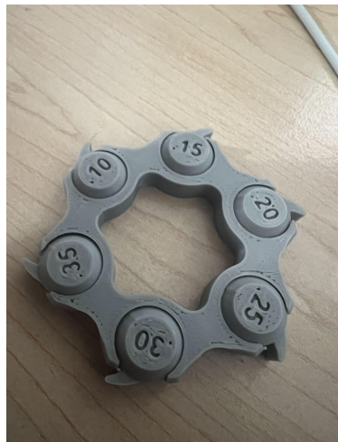
Figure 12.1 - Tolerance test print
